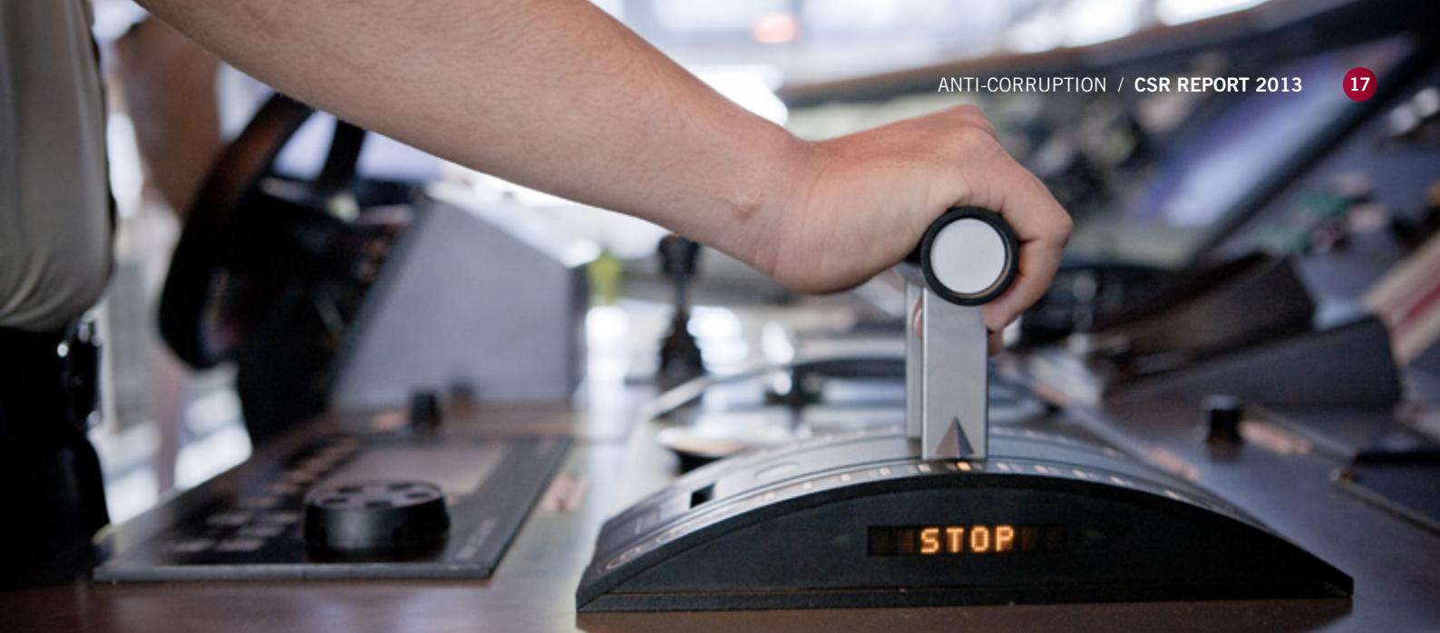
The engine-telegraph on the bridge of the dry cargo vessel NORD AQUILA.
