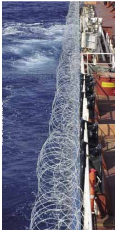
NATO razor wire is one of the measures to prepare a vessel for transit through the Gulf of Aden.
