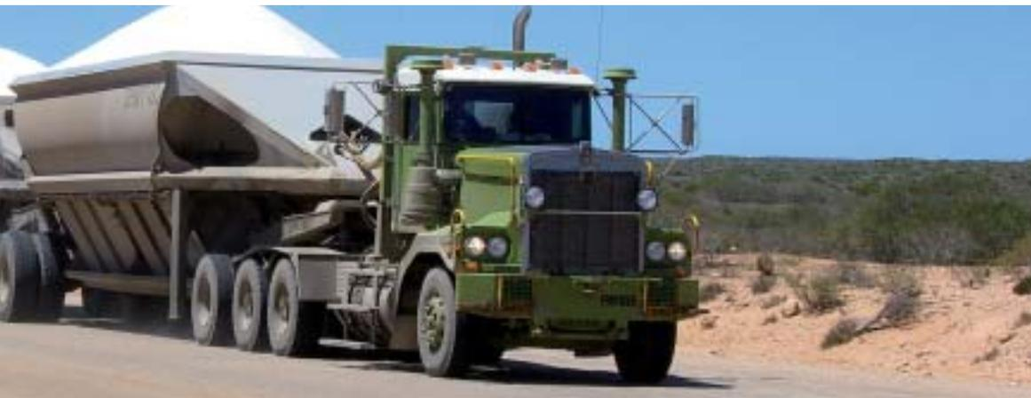
WHEN THE SALT HAS BEEN WASHED, IT IS TRANSPORTED TO THE VESSELS IN LARGE TRUCKS. THIS TRUCK HAS A CAPACITY OF 1,000 HORSE POWER AND CARRIES APPROX. 250 TONNES IN FIVE VEHICLES.
