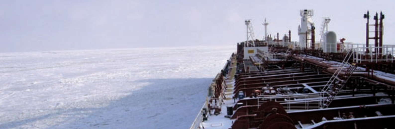
FIRST-YEAR ICE: THE ICE IS FORMED DURING ONE WINTHER AND HAS A THICKNESS OF MORE THAN 30 CM
