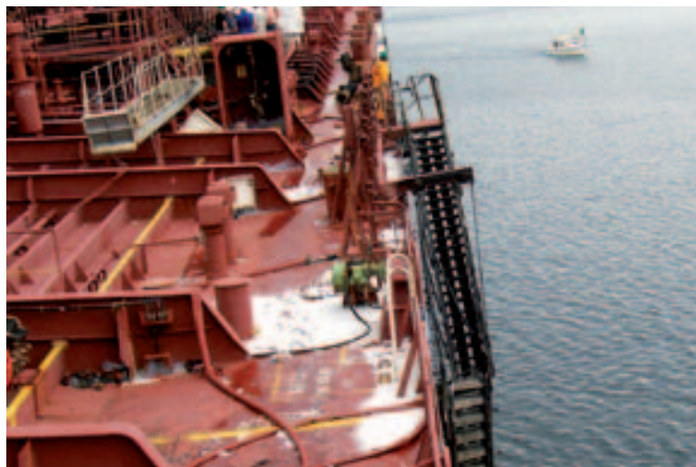
THE GANGWAY WAS TORN APART WHEN THE M.T. NORDEUROPA PULLED AWAY FROM THE QUAY. THE FIRE FIGHTING FOAM ON THE DECK IS EVIDENCE OF THE FIRE.
